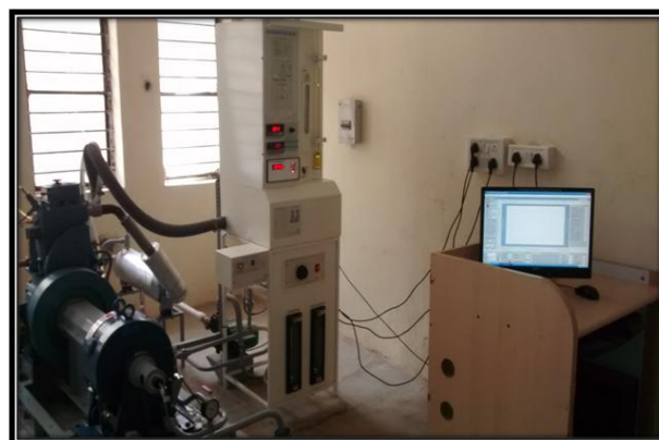
Figure 2: Computerized research diesel engine set up
